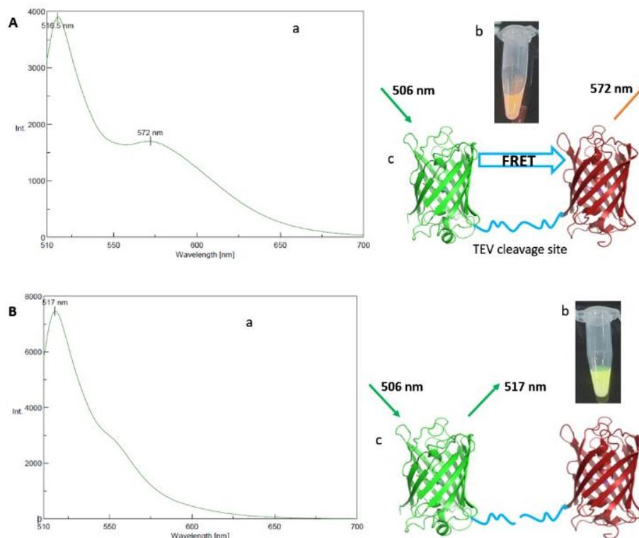
Figure 5 A. Images of the produced mNG-TEV-mRuby3 FRET sensor. Emission wavelength graph of the produced FP-FRET sensor (a), image of the FP-FRET sensor under UV light (b), schematized version of biosensor (c). B. Images of the mNG-TEV-mRuby3 FRET sensor after the TEV protease activity. Emission wavelength graph of the FP-FRET sensor after protease activity (a), image of the biosensor under UV light after the TEV protease activity (b), schematized version after the TEV protease activity (c).
