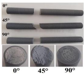
Figure 9. Tensile test samples fracture surfaces
