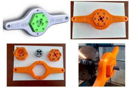
Figure 3. Design and produced novel threading tool
