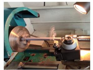
Figure 2. Turning process for 3D printed bolt shafts
