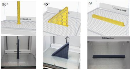
Figure 1. G code view and produced bolt shafts
