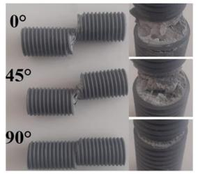
Figure 10. Shear test samples fracture surfaces
