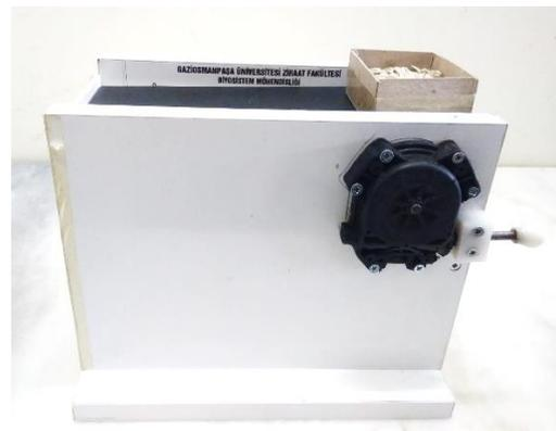
**Figure 3.** Static friction coefficient measurement
