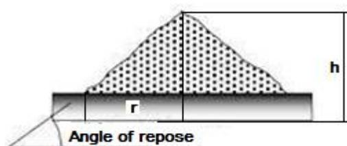
Figure 4. Measurement of the angle of repose
