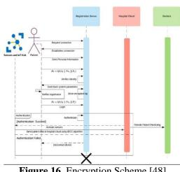
Figure 16. Encryption Scheme [48]
