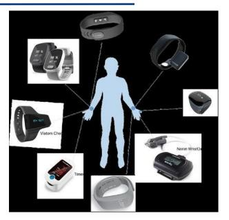
Figure 2. Wearable pulse oximeters [8]
