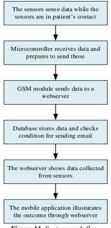
Figure 11. System work flow
