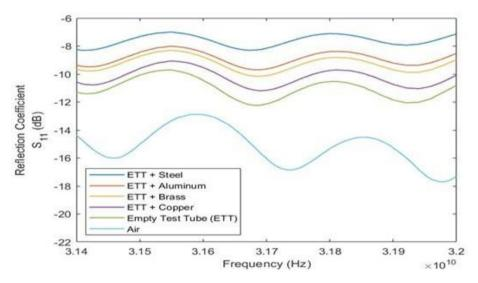
Figure 4. Reflection coefficient data obtained using empty container and reflective materials at 31 GHz.
