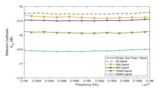
Figure 5. S<sub>11</sub>-reflection coefficient data obtained using the WR-28 adapter and steel
