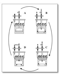
**Figure 4.** Technological design and operating principle of the RITA system: (A) exposure time; (B) Displacement of the liquid medium. Air pressure is applied to the lower chamber through the middle pipe. Liquid media moves to the upper chamber; (C) immersion time; (D) evacuation of the nutrient medium. The airflow is stopped and the medium flows back into the lower chamber due to gravity.
