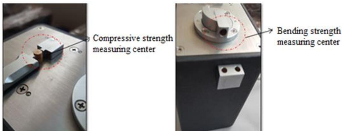
Figure 2.6. Bending and compressive strength measuring device
