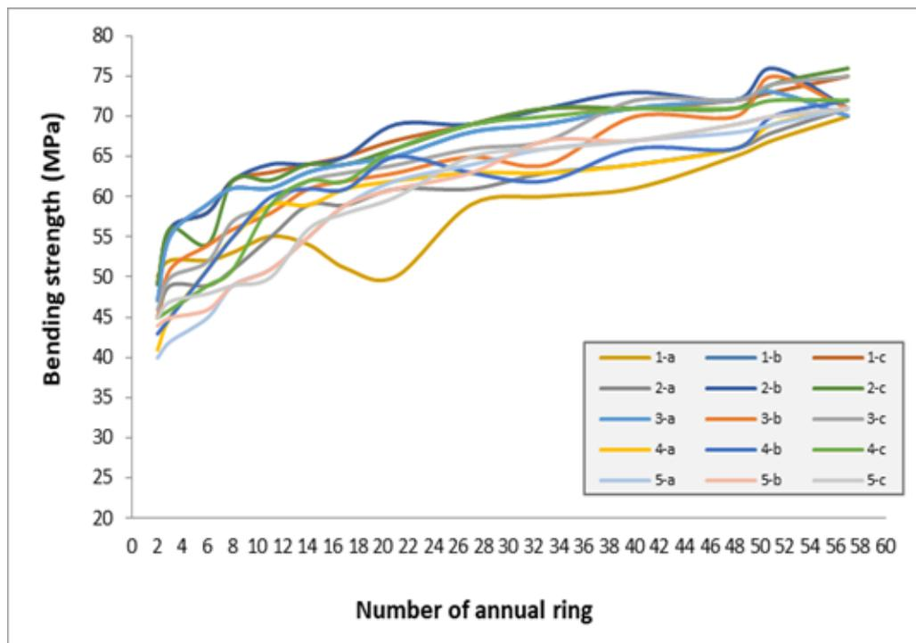
Figure 3.5. Bending strength values based on annual ring
