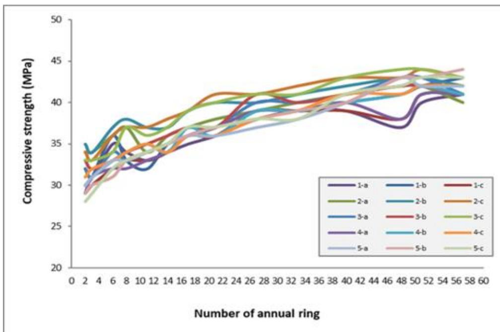
Figure 3.4. Compressive strength values based on annual ring
