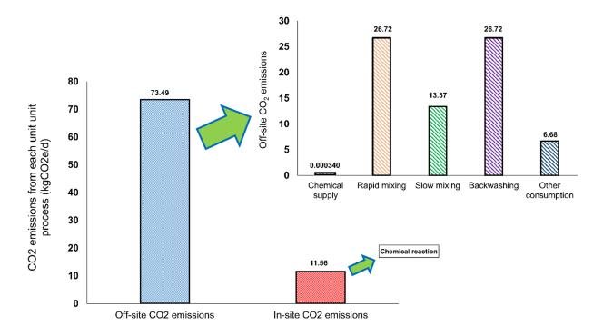
Figure 2. The CO<sub>2</sub> emissions from each unit process of the drinking water treatment plant
