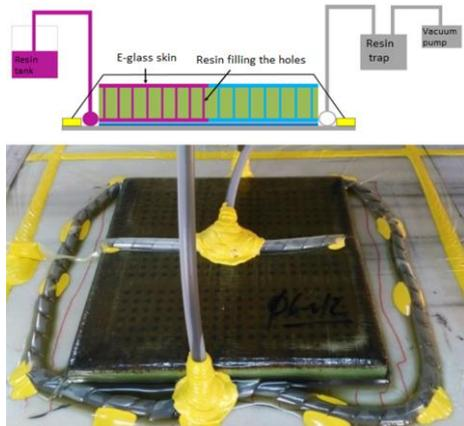
**Figure 2.** Production of pin reinforced sandwich panels
