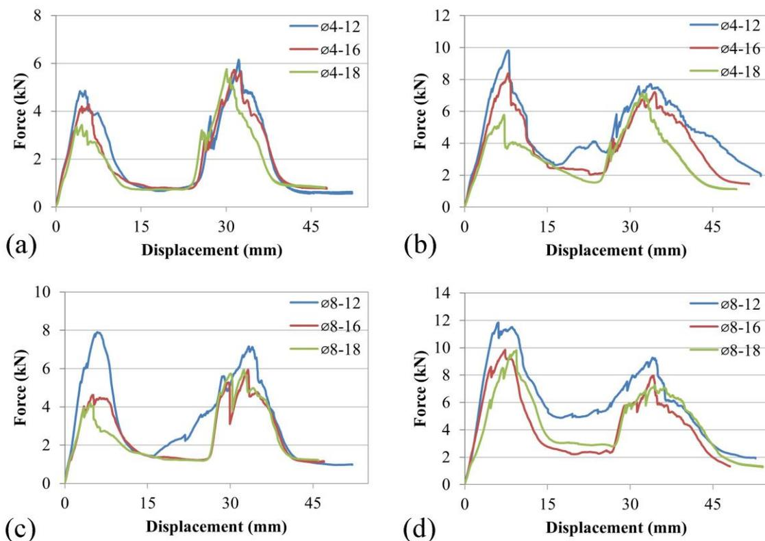
**Figure 4.** Force-displacement graphs of sandwich specimens, with  $\text{Ø}4$  mm diameter pins tested with (a)  $\text{Ø}12.7$  mm and (b)  $\text{Ø}20$  mm indenters, with  $\text{Ø}8$  mm diameter pins tested with (c)  $\text{Ø}12.7$  mm and (d)  $\text{Ø}20$  mm indenters
