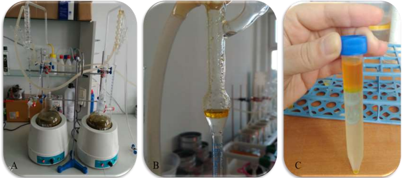
Figure 1. S-H Clevenger equipment (A) collection of black cumin oil (B) and black cumin oil transferred into the falcon tube (C)
