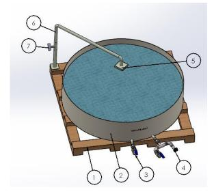
Figure 2. Location of the ultrasonic sensor on Class A pan
