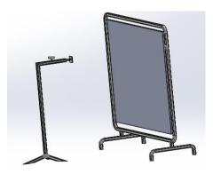
Figure 7. Sensing range adjustment board for ultrasonic sensor
