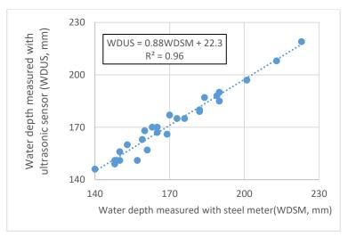
Figure 9. Water depth values measured in Class A pan with steel meter and ultrasonik sensor
