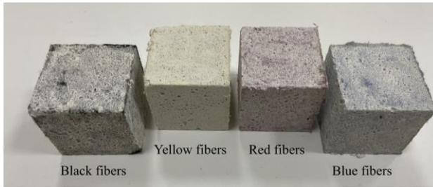
Figure 1 Mortar specimens produced using different colored fibers
