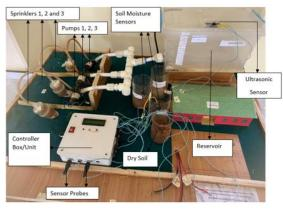
Figure 5. Laboratory-scale smart irrigation test-bed (Ogidan et al., 2019).
