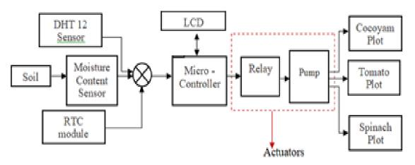
Figure 1. Block diagram of the smart irrigation system based on crop water use.
