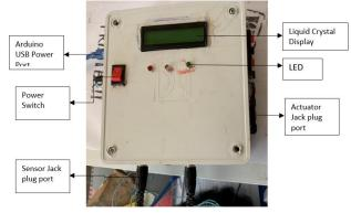
Figure 4. Developed system after coupling.
