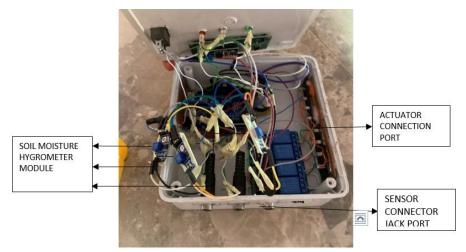
Figure 3. System being coupled.
