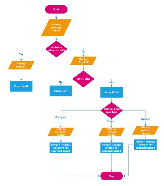
Figure 2. Flowchart of the smart irrigation system based on crop water use.
