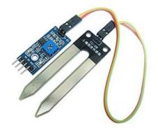
Figure 6. Soil moisture sensor.
