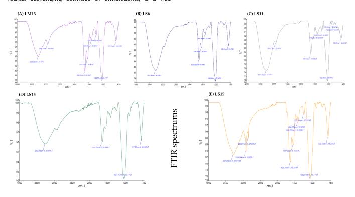
Figure 1. FTIR spectra of the EPS samples (in the range of 400–4000 cm<sup>-1</sup>)
