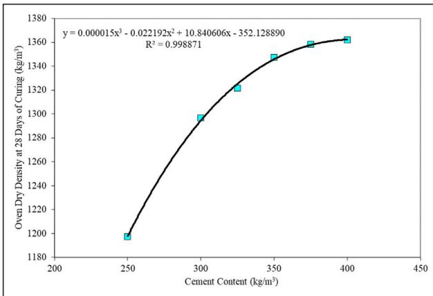
Figure 3. Cement amount versus density of concrete.
