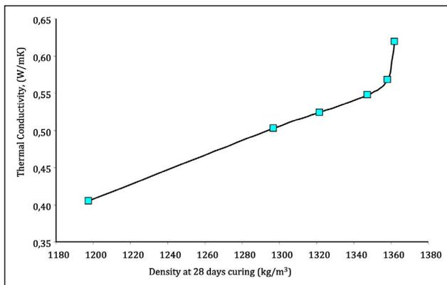
Figure 7. Density versus thermal conductivity of concrete.
