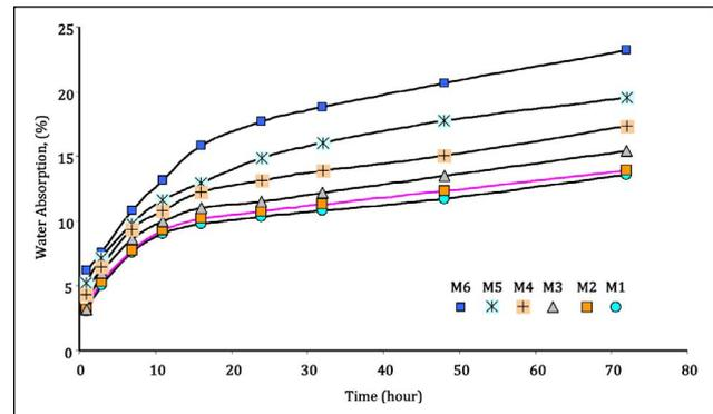
Figure 6. Water absorption versus time for PARLC samples.
