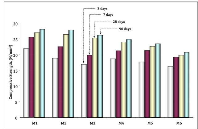
Figure 4. Curing time versus compressive strength of concrete.
