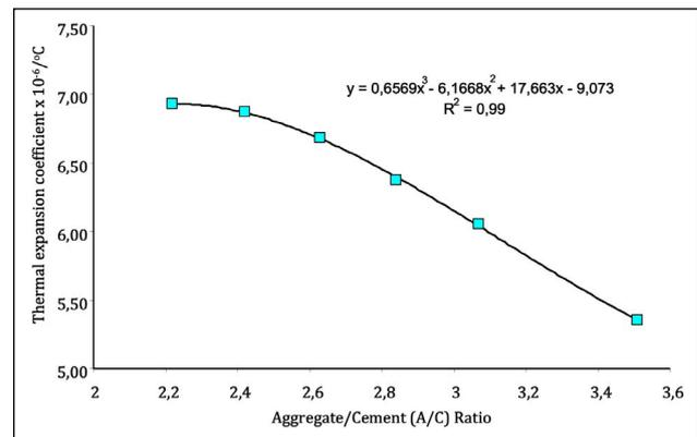
Figure 8. A/C versus thermal expansion coefficients of concrete.
