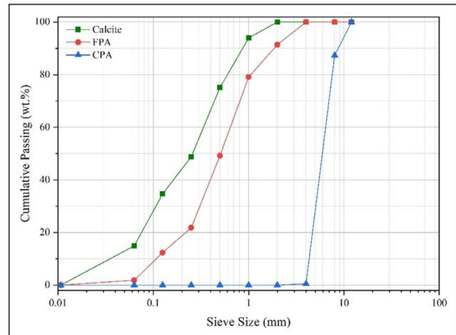
**Figure 2.** Sieve analysis of calcite, FPA, and CPA.
