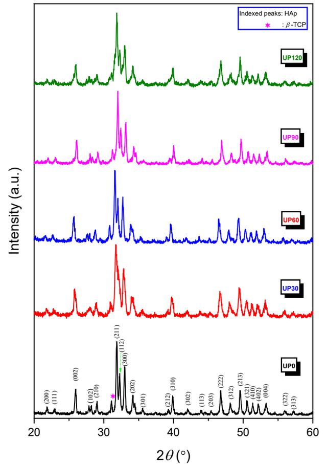
Fig. 1 XRD patterns of the as-synthesized HA samples
