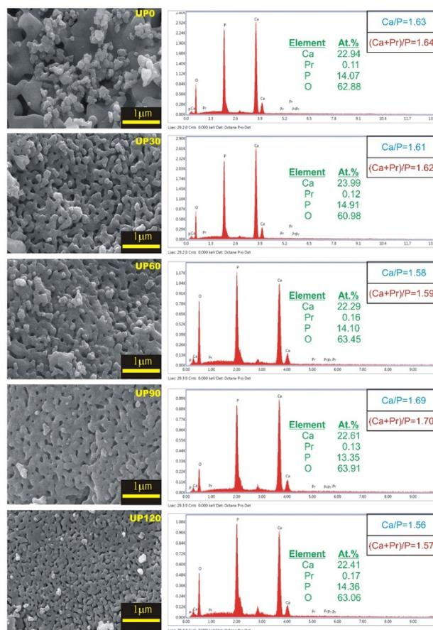
Fig. 3 SEM observations with the EDX analysis results
