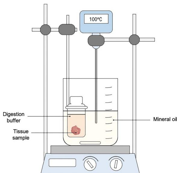
**Figure 1.** Wet digestion set up for breast tissue samples.**Table 1.** Operating conditions of the ICP-MS
