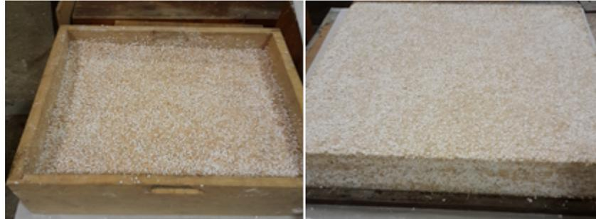
Figure 1. Polystyrene composite particleboards draft
